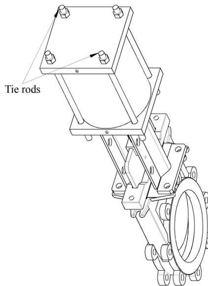
**Figure 3: Cylinder-operated valve**
