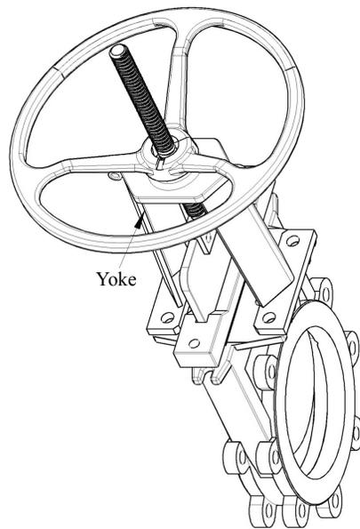
**Figure 1: Handwheel-operated valve**
