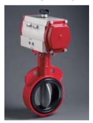
**DIRECT MOUNTING** Bray actuators comply with ISO 5211 dimensions and mount directly to Bray valves without using external linkages. Field installation is simple, misalignment is minimized and contamination buildup between valve and actuator is reduced. Bray can provide linkage for mounting actuators to other devices requiring 90° to 180° rotation.
